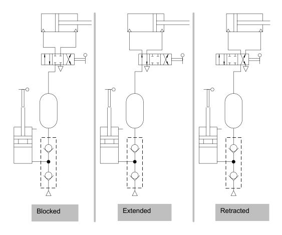
These three circuit diagrams correspond to the model states, depending on the position of the manual valve. We will be explaining the circuit symbols using the drawing at the left called "Blocked":
