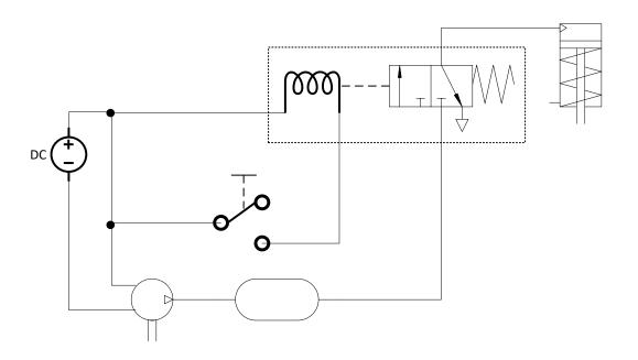
The power supply (at the left of the circuit diagram) is shown here as well, since it is required to connect the button and solenoid valve.
