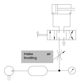
b) However, we can also throttle the *exhaust*: We allow the intake air to flow into the cylinder unthrottled, but use a throttle to prevent the exhaust on the other side from flowing quickly out of the cylinder.
