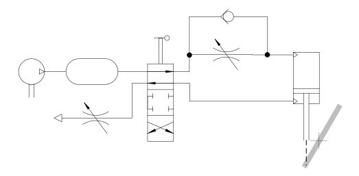
When the barrier is closed, both throttles act in a series:
