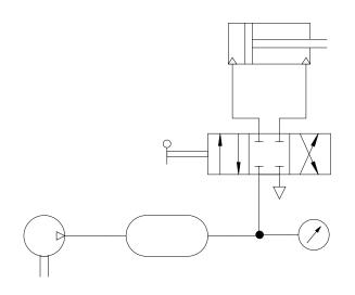
The left element stands for the compressor. Its power supply is not separately shown. The circuit symbol for the manometer to the right of the air tank is also new.
