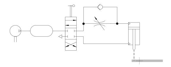
We are using one throttle in the hose between the valve and the top end of the barrier cylinder. When the barrier closes, the cylinder retracts, and the exhaust on its upper connection in the barrier model must be throttled.
