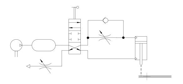
However, the stronger throttle is the only one that is primarily active. With this circuit, you can throttle closing of the barrier more than opening, but not vice versa. If you want to do the opposite, the throttle/check valve combination would have to be connected to the other cylinder connection.
