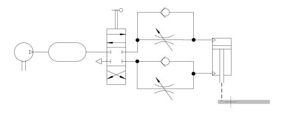
Both of the check valves must be installed so that they throttle the exhaust, but not the intake air.
