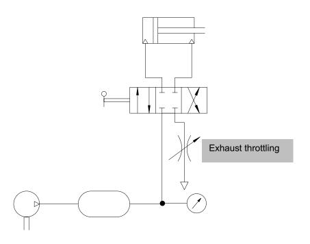
Let's try it! Add the throttle to the expanded functional model. It is simple to use: Insert a hose through it; then you can turn the blue handle to screw in a screw. This will press on the hose and allow you to finely adjust the "remaining" diameter of the compressed hose. We will be testing out both the intake air and exhaust air throttling in this way.
