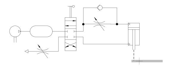
When the barrier is opened, and the cylinder extended downward, the intake air on the cylinder would not be throttled due to the check valve, but the exhaust would very likely be throttled at the bottom connection – see the following valve position:
