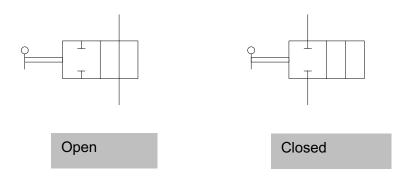
We do not put an arrow in the box for the connected switching position, since without the context of the whole circuit diagram there is no definition of which direction the air would flow through the valve, and because the hose does not have any design restrictions on the flow (the air can simply move through in both directions).
