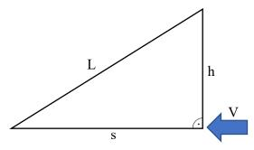
L is the length of the bar, the lower end of which is away from the cylinder. s is the length of the projection of L on the plane. h is the stroke (here measured from the plane). L, s and h form a right-angled triangle.
